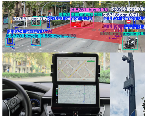
Elements for protecting VRUs include detection by cameras, roadside infrastructure and an HMI inside the vehicle
